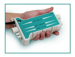
The **ViP Ventilatortester** is a mobile microprocessor controlled measurement meter for flow, volume, pressure and oxygen. Developed for medical and laboratory applications and especially used to test ventilators its main advantages are its high measuring precision and simplicity of use. Its wide spectrum of use lets this meter stand as an ideal unit for surveying and testing tasks. The measured values can be displayed, saved and printed by a PC programme (communication via RS232).
