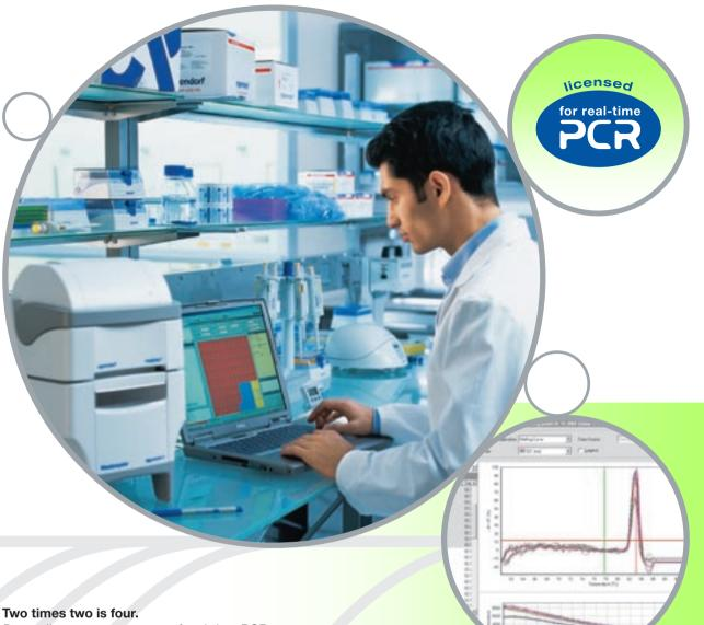
Depending upon your range of real-time PCR applications, select between two available detection systems — Mastercycler ep realplex² and Mastercycler ep realplex⁴. Both are operated by the same realplex software, and both are equipped with an LED array to excite the fluorescent dyes in each individual PCR sample. The differences between each system include the number of fluorescence filters and photo-multipliers and the different, resulting levels of multiplexing capacity.
