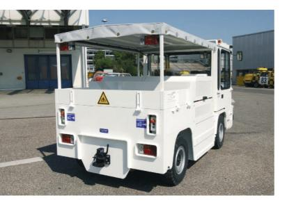
Powered by hydrostatic transmission, this Rofan tow tractor combines the power and reliability of a diesel drive with the economic efficiency and environmental friendliness of an electric engine.
