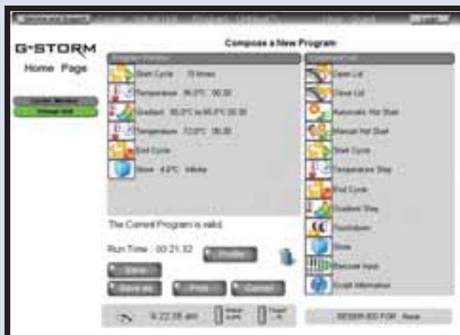
■ The icon driven, drag and drop programming is simplicity itself. Simply select the command that you require, drag it into the program window and enter your parameters when prompted. This method enables both complex and simple protocols to be visualised during programming by selecting the "profile" option.
