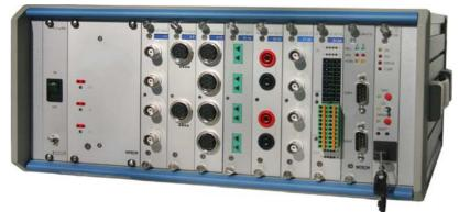
rates of the amplifiers are up to 20 kHz per channel. AD conversion is done with 24 bit resolution, digital data output with 16 bit. Calibration data and the complete parameter settings are stored in a flash EPROM. All channels are isolated and work synchronous.
