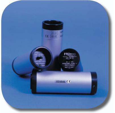
A range of adaptors is available which allow the units to be used with a wide range of different microphone capsules. As standard, the units are provided with a QC:3 <sup>1</sup>/<sub>2</sub>" adaptor. Please refer to the specifications overleaf for details of the available adaptors.
