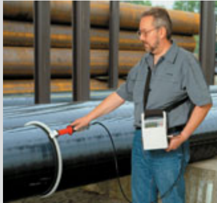
Porosity detection on pipelines
