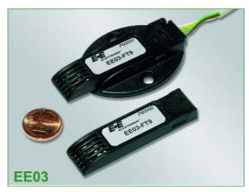
The EE03 features an embedded microprocessor that retains calibration data, and provides a full-range, temperature corrected humidity output. The simple E2 digital protocol used by the EE03 allows for low-cost integration with other devices utilizing microprocessor based control or monitoring.
