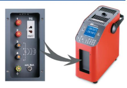
Resistance thermometers, thermocouples, temperature transmitters and switches must be operated in the calibration with a measuring instrument which measures and displays as temperature the output signals such as resistance values, thermal voltages and norm signals.
