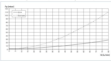
The diagram shows exemplarily the pressure loss characteristics when air flowing through.
