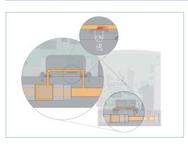
The actual flow rate is detected by a sensor. This operates according to a thermal principle which has the advantage of providing the mass flow which is independent on pressure and temperature.
