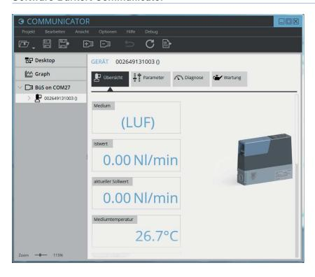
Part of Bürkert's new EDIP program (Efficient Device Integration Platform) is the Bürkert Communicator. This software can be run under MS-Windows and allows users to program further parameters in MFCs or watch process controls. It is freely available on Bürkert's website. An accessory part, the büS stick – please see ordering chart for accessories, serves as the interface between computer and process instrument I want to connect to. It transfers "USB data" to "CAN data". The Communicator allows:
