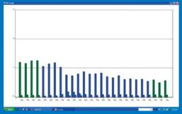
UV monitoring data of a 26-mer peptide using feedback control to increase the number of deprotection cycles and modify the subsequent coupling cycles.
