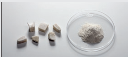
Bone material before and after grinding with the FRITSCH PULVERISETTE 0
