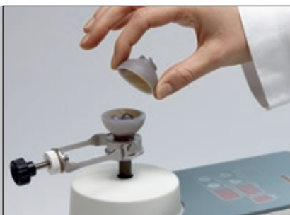
Practical and effective: Spherical grinding bowls for easy assembly
