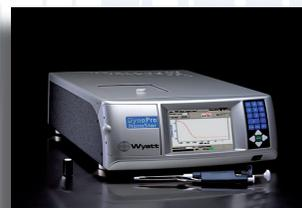
18-angle MALS light scattering detector for the measurement of absolute molecular weight, size, and conformation of macromolecules in solution.
