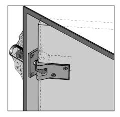
At least two hinges are necessary per door. They should be mounted at approx. 60 mm (for 4000 and 4500 models) or 120 mm (for 40K, 41K, 41, 42 models) below the upper edge or above the lower edge of the door leaf.
