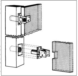
ATTENTION: if the holes fixing the shoe to the door are not exactly central to the holes in the shoe, the shoe could become slightly distorted and get jammed against the spring.
