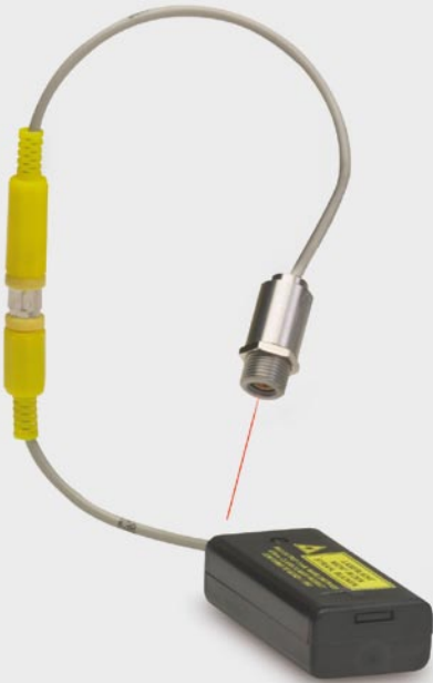
TM-LST-CT Laser-Sighting tool
