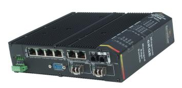
Magnum™ 6KQE Managed Edge Switches provide configurability in an entry-level industrial-grade package. The high performance 6KQE base unit comes with four 10/100 copper ports (which may be either regular or PoE). Up to 3 100Mb fiber ports or up to four more 10/100 copper ports, or combinations, may also be configured. In addition, one or two Gb ports may be configured as 10/100/1000 copper or SFP fiber in any 6KQE base unit.
