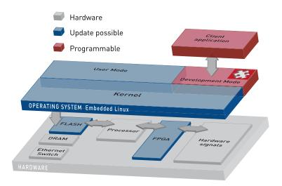
The MSX-E modules are organised in two levels: the hardware and the software level. The control part of the hardware [ARM9, Flash, etc.] is common to all module types. The signal part features the specific function of each module type: counter, digital I/O, analog I/O, length measurement, etc. The Embedded Linux operating system is saved in the FLASH and is loaded at booting through the ARM9 processor into the RAM and FPGA.
