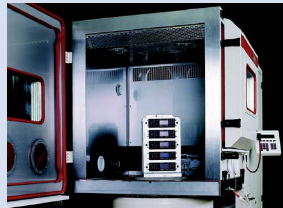
Combined climatic and vibration testing of car radios at Blaupunkt GmbH, Hildesheim/Germany
