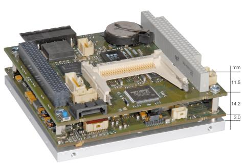
MIP10 dimensions 96 x 90 mm therefore fully PC/104-Plus compliant
