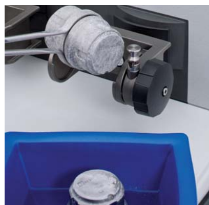
Before grinding, the jars are immersed in liquid nitrogen (-196 °C) in the cryo box for approx. 2 - 3 minutes
