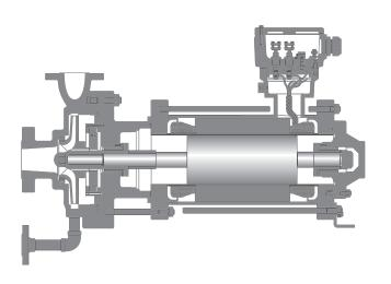
Single-stage canned motor pumps in process design according to API 685
