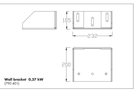
Use of the wall bracket r 0,37 kW: - DICTAMAT 900-21, 0,37kW door operator
