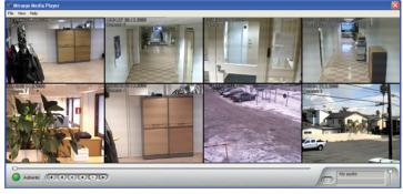
Mirasys Media Player can be used to play media clips. The clips can contain data from up to 8 video and/or audio channels. All data can be played synchronously. Single images can also be printed. In addition, the player verifies the authenticity of the media clips. The player is automatically exported with media clips and saved to the same folder as the clip.
