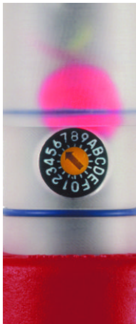
16-position rotary switch for set point adjustment
