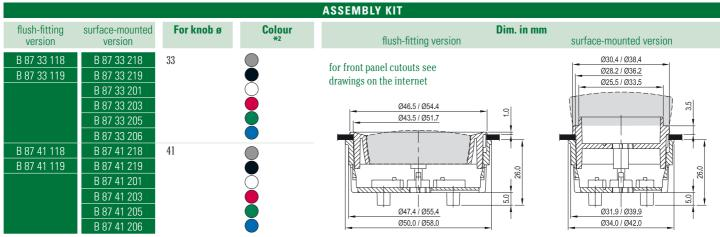
Minimum components for 1 STAR-KNOB: 1 knob, 1 cover and 1 assembly kit.
