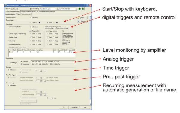
Besides the amplifier-selectable levels, further trigger conditions and combinations of digital and analog values can be set in DAQSoft, as well as time-trigger points and parameters for periodical respectively recurring measurements.
