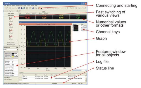
Activating the TCP/IP connection and pressing the start button will start the measurement. Selected channels will be automatically displayed. The dockable windows for views, values, graph, features, log file, etc., can be arranged any way or faded in and out.
