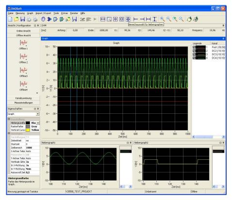
All channels can be displayed in the main graph, but also single or grouped in side graphs. For a higher resolution a different time base compared to the main graph can be chosen; the Y axis however has the same scale. This presentation works in online and offline mode.
