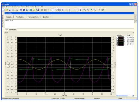
Besides the comparison of signals, the combination and mathematical post-processing of channels is possible. Also post-filtering of channels as well as analysis with FFT or power spectrum can be realised.
