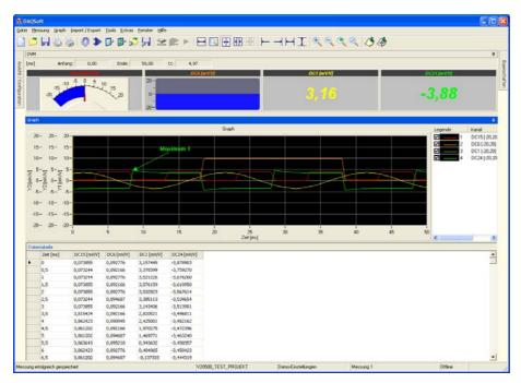
Minimum and maximum values can be analysed in offline mode and documented with an annotation. Parallel to the numerical and graphical presentation of the values, a visualisation in tabular form is possible.
