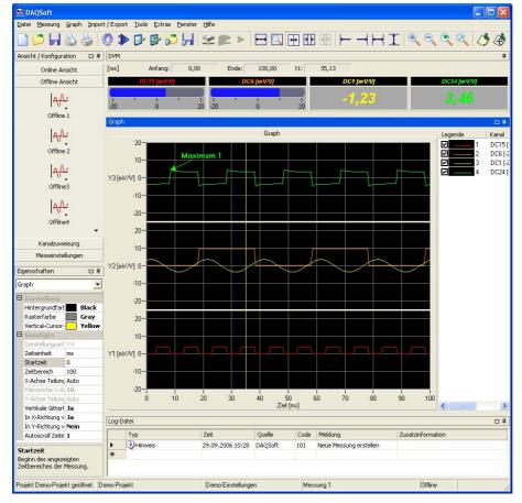
Alternatively the signals can be displayed in stacked plots. All stacked plots have a common time axis; the Y axes can have individual graduations. The measurement values can be displayed numerically, or in bar respectively round reading instruments.
