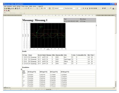
DAQSoft also has an export function for its measurement data into other formats like Famos, DIAdem, MATLAB, and ASCII. Further on reports for reading in Internet Explorer, Word or Excel can be generated. These reports can be adapted individually for heading, graphical display and selected data.
