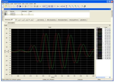
Direct comparison of signals is also easy in offline mode. By entering time offset values, signal curves can be shifted against each other any way.
