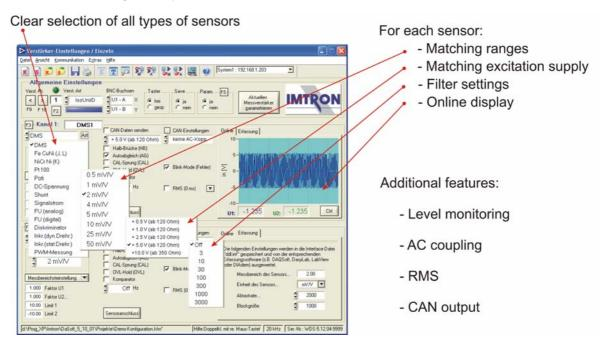
Parameter setting is done by channel or table-driven in DaSoft. After selecting the type of sensor, the corresponding measurement range is set, and if necessary excitation voltage as well as cut-off frequency. Checking of the signal is done using the online display.
