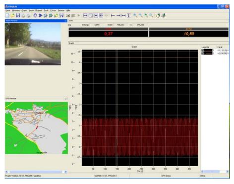
An extended version of DAQSoft acquires GPS and video data via suitable hardware synchronous with other measurement data. This allows optical and spatial coordination of events.
