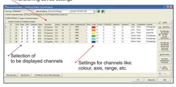
Parameters set with DaSoft are automatically taken over by DAQSoft. Now the to be displayed and saved channels can be selected, and their settings like colour, axis, range be fixed.
