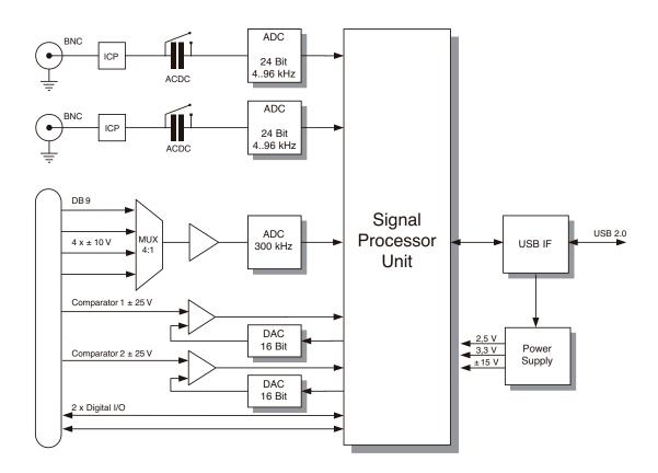
The main inputs of the RogaDAQ2 are simultaneously sampled precision analog inputs for recording dynamic signals. Sampling rates up to 48 kHz at up to 24 Bit resolution are supported. Each channel features instrumentation quality preamplifiers, AC or DC coupling and constant current sensor supply for directly supporting IEPE—type sensors.
