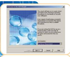
Set up your Standard Operating Procedure (SOP) using the system's integrated method definition wizard. SOPs lock-down all aspects of the measurement process including the hardware configuration, analysis settings, triggering options, result parameter reporting and data averaging. Online help supports method specification for different spray types.
