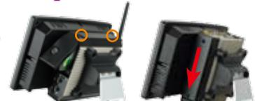
Screw to fix uIBX-200. As different applications, the direction of assembling can be changed.
