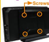
Install the mount kit in back of monitor.
