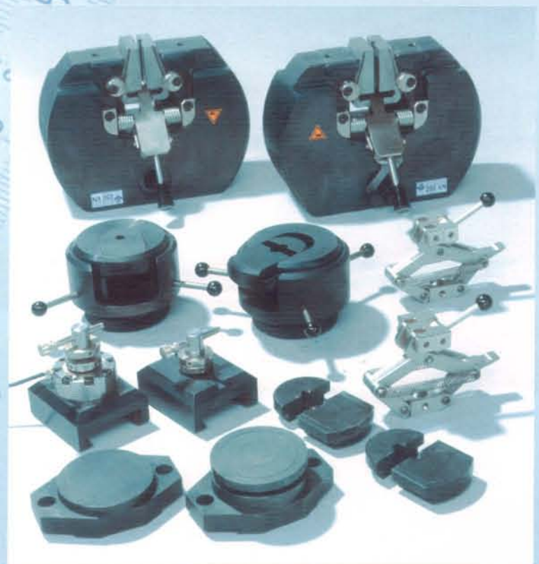
Wedge type grips 100 kN with insert system for additional clamping tools
