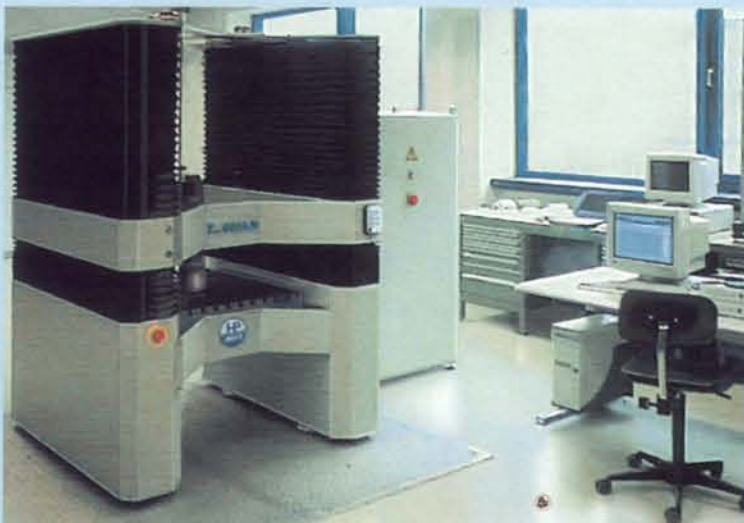
Inspekt 600 kN PUM.A universal testing machine with four separate drives and screws for simulating molding processes
