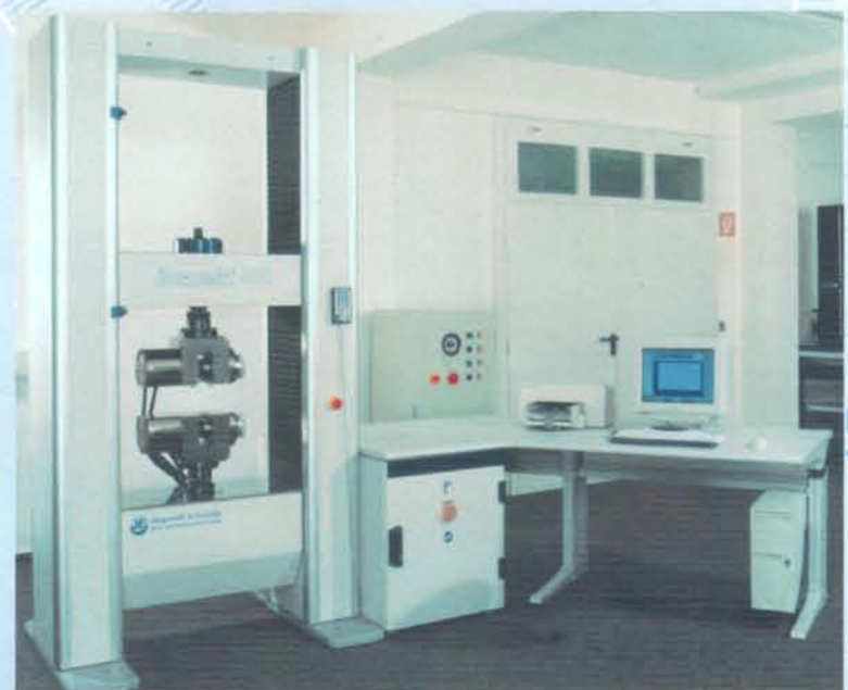
Universal Testing Machine Inspekt 400 with hydraulic clamping tools
