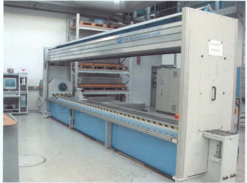
Inspekt 600 kN-L horizontal testing machine for testing high-current insulators, machine fully enclosed with roller doors
