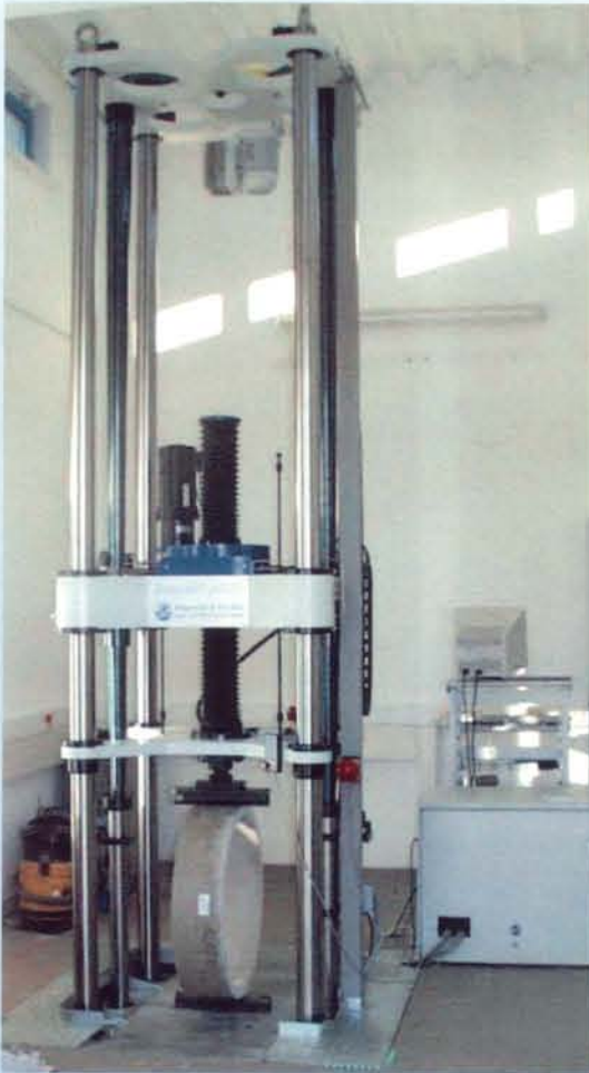
Inspekt 500 kN universal testing machine for apex (vertex) pressure testing on fibreglass compound pipes with a maximum diameter of 3000 mm
