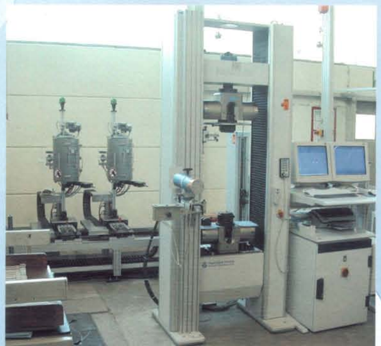
Hot tensile testing system for high temperature application
