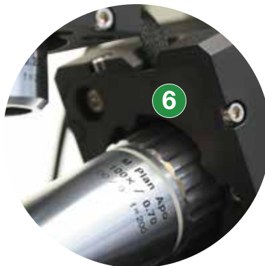
Closed-loop, short path-length Raman laser alignment for long-term stability
