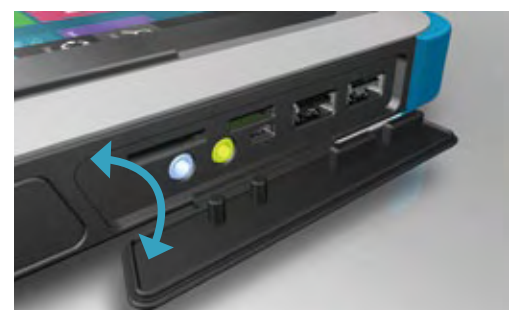
A special protective cover is designed to prevent water and dust from entering the device.
