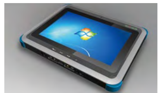
Protective rubbers are located on all four corners of the ICEROCK3, enhancing its strength against bumps and drops.
