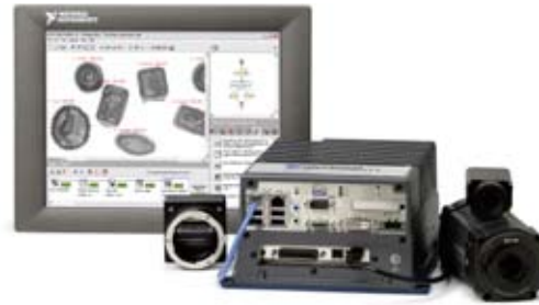
Figure 2. You can configure the EVS-1464RT using Vision Builder AI or program the system using the Vision Development Module.
