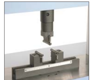
3-point bending test of plastic specimen
