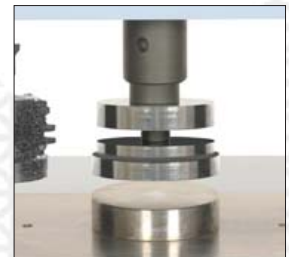
Spherical seat type compression plates
