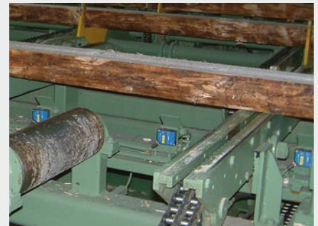
optoNCDT on trimming systems of saw mills
