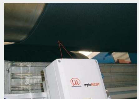
High speed measurement of black rubber
