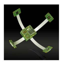
Up to four pixel-synchronous CMOS sensors with global shutter can be connected to the central unit of the multi-sensor camera by an LVDS data cable and can be freely positioned. The image data is coordinated on a FPGA module with at least 256 MB RAM. The multi-sensor camera is available in colour or monochrome, and optionally with lenses ("Cob" variant).
