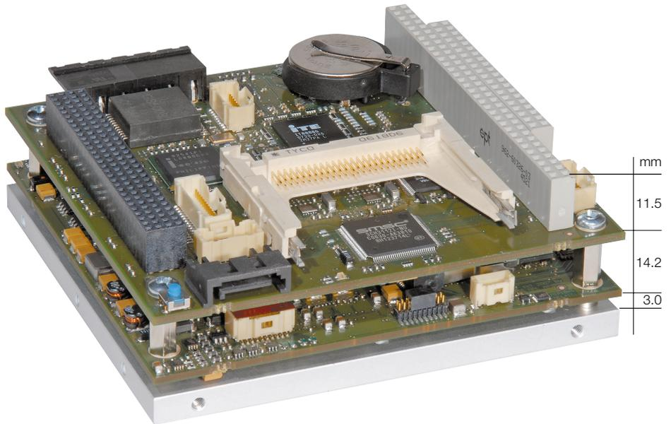
MIP10 dimensions 96 x 90 mm therefore fully PC/104-Plus compliant
