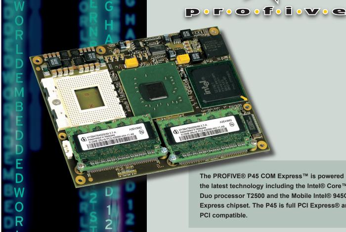
The PROFIVE® P45 COM Express™ is powered by the latest technology including the Intel® Core™ Duo processor T2500 and the Mobile Intel® 945GM Express chipset. The P45 is full PCI Express® and
